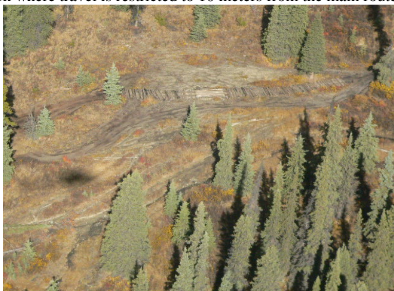
Figure 18: Corduroy constructed trail route.
